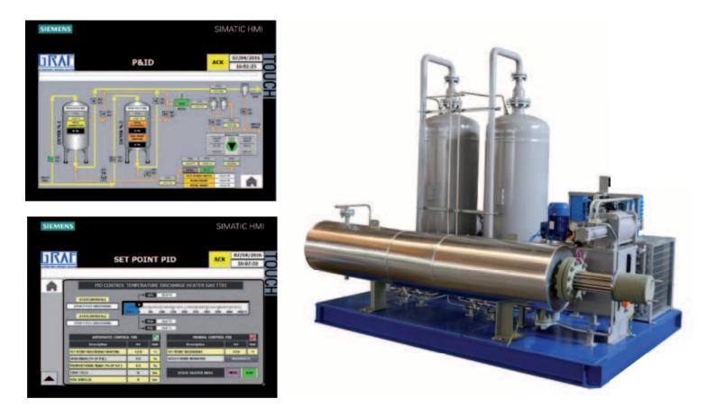
GRAF **regenerative** type dryer series **GRGDR** is composed of two columns filled with molecular sieve and is completed with an automatic closed loop circuit regenerative system with no gas emission.
